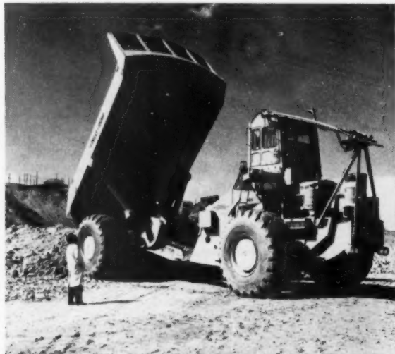
DIESEL ENGINE supplies power to wheel motors when truck is away from trolley power at loading and dumping areas.
